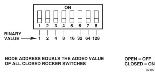
Figure 18—Address Switches for Detector
