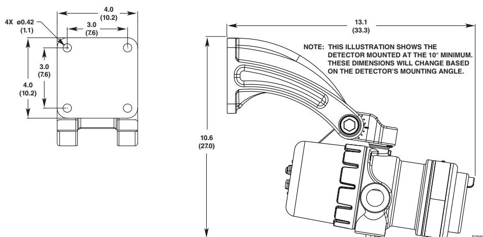
Figure 3—Q9033 Mounting Arm without Collar Attachment Dimensions in Inches (cm)
