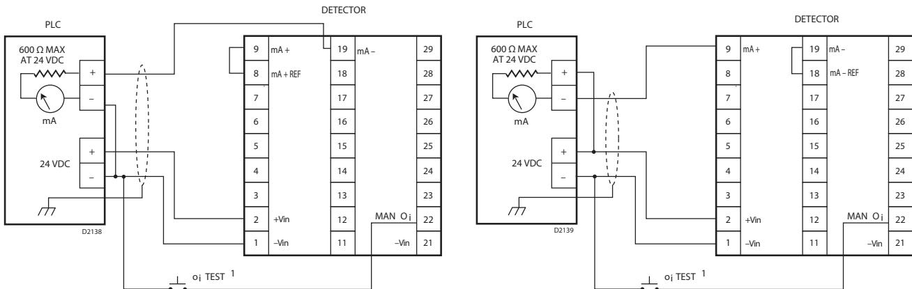
Figure 10—Detector Wired for Non-Isolated 0 to 20 mA Current Output (Sourcing)
