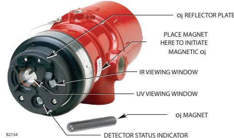
Figure 2—Front View of the Detector
