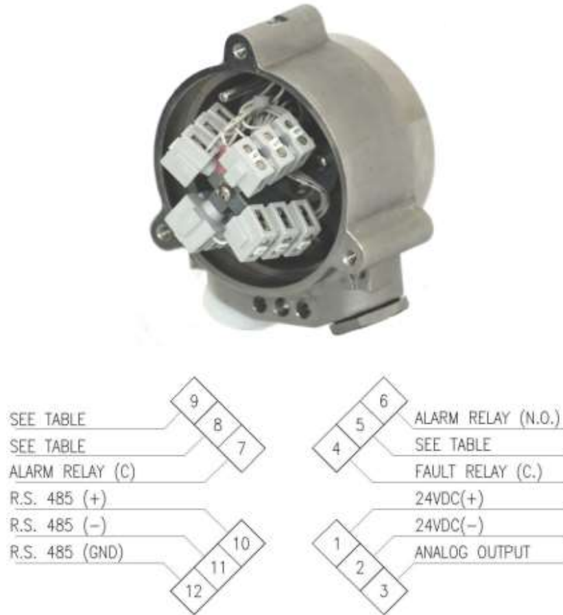
Figure 8: Wiring Terminals
